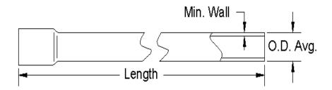
National PVC TELE-DUCT is manufactured from virgin PVC compounds with a cell class of 12454-B as determined by ASTM D-1784. The materials used and methods of manufacturing, testing, handling, and shipping, shall be such as to insure a quality finished product.
